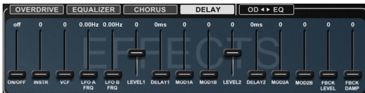
This is a tape-style delay. Unlike the Chorus, here the delay lines are much “darker” than the dry signal due to having a greater proportion of the high frequencies filtered out. It is a classic effect often used with synthesizers..
