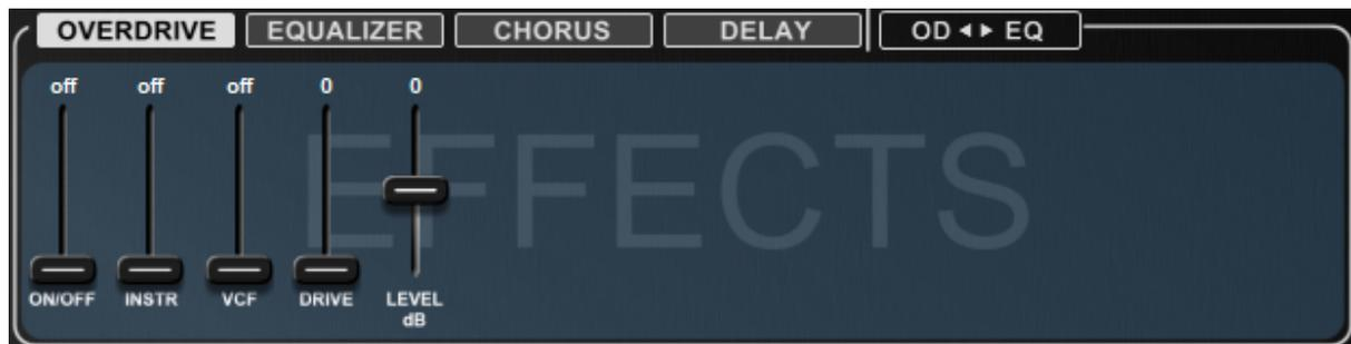
At lower levels, you can use this effect to create sounds that emulate the warmth and breakup of a tube amplifier. At higher levels you can create some quite grinding distortion sounds.
