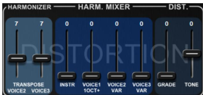
The Distortion Block applies distortion to the original instrument signal and to the three transposed voices generated by the Harmonizer.<sup>16</sup> VOICE1 is fixed at 1 octave above the input signal, whereas the transpositions of VOICE2 and VOICE3 are variable.
