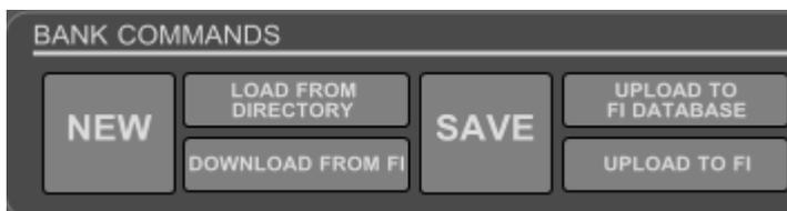
The buttons of this section control various aspects of the tiles of the Tile Window that correspond to the 99 memory slots of the FI4. The tiles are used to transfer programs between your computer and the FI4, save them to your computer or upload them to the Online Program Database.
