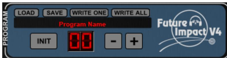
This area in the upper-left corner of the Editor is used to show the currently-loaded sound. The name and category is shown in the long window. The faux-digital window shows the program number (but is blank if the program was loaded via the [Manager's](#) Tile Window).
