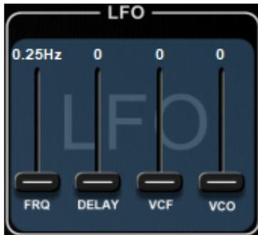
The FI4 has a dedicated Low Frequency Oscillator (LFO) for modulating the cutoff frequency of the VCF and the pitch of the VCOs. This can be used to create pitch vibrato and filter “wobbles”.
