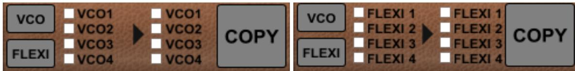
In the lower-left corner of the Editor there is a tool to copy all settings of one [VCO](#) (oscillator) to one or more of the other oscillators or to copy all parameters of one [Flexi Controller](#) to one or more of the other Flexi Controllers.
