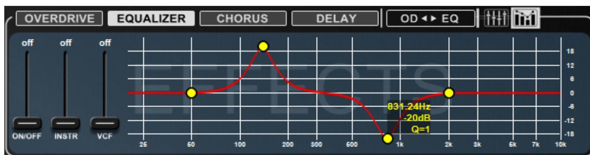
This block contains four effects: [Overdrive](#), [Equalizer \(EQ\)](#), [Chorus](#) and [Delay](#). Up to three of the effects can be used simultaneously, though **Chorus and Delay cannot be used together**. Chorus or Delay is fixed at the end of the chain but the order of the other two can be changed at will. The effects are fed by the INSTR and VCF outputs from the Main Mixer.
